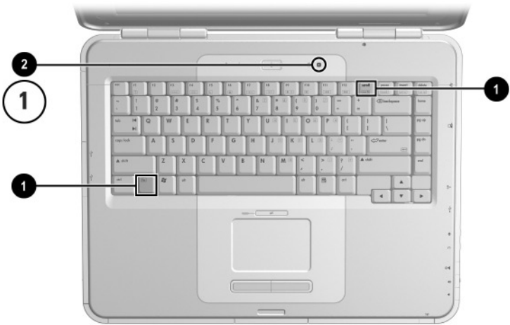
Identifying the Fn and num lock keys and the num lock light
