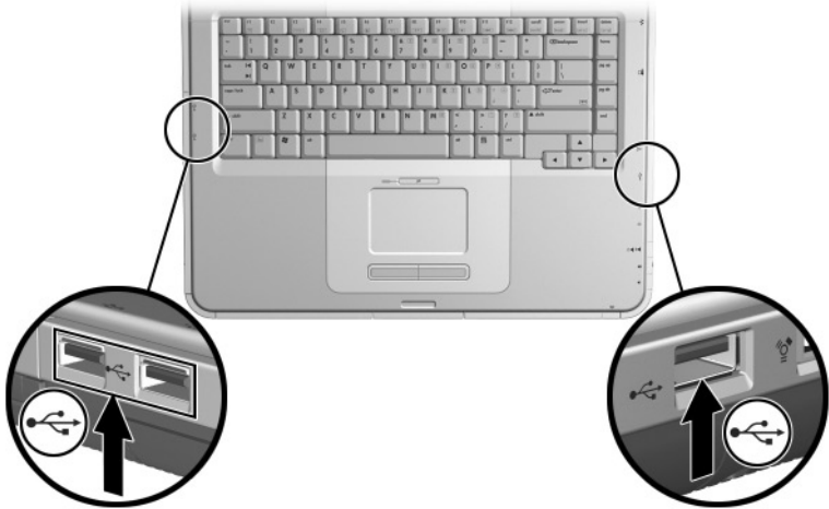
Identifying the 2 USB connectors on the left side and one USB connector on the right side
